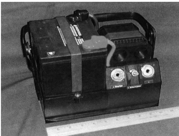
Fig. 7. 12-V dual-battery system.
